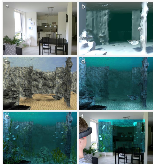
Fig. 1: Creation of the mixed-reality world: a) the user's real environment b) the reconstructed surface of the real environment c) virtual models based on the reconstructed surface (using textures) d) with underwater lighting simulation e) with added animals and plants f) illustrating the user's perspective.
